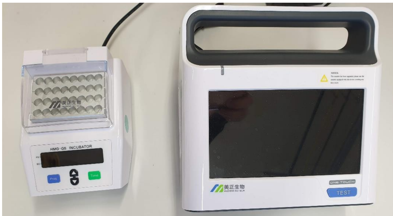
Fig. 2. HMG-GS Microwell Incubator and BMZ6000 Portable Strip Reader for instrumental reading of the color formation on the AnticFast® Beta-lactams & Tetracyclines & Cefalexin Rapid Test Kit test strips.
